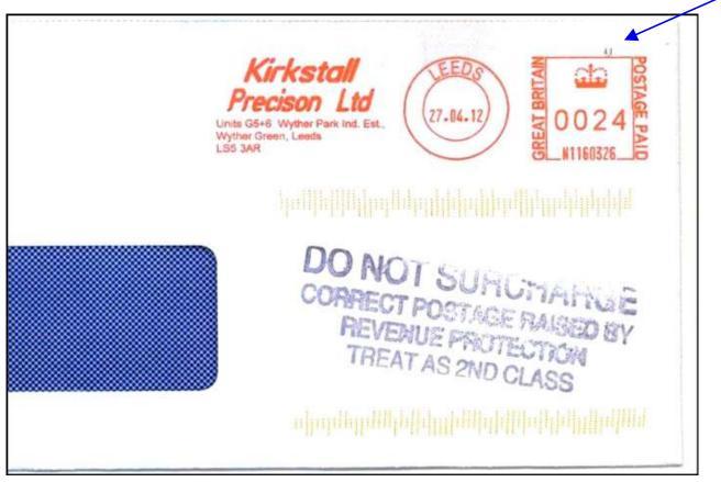
The Royal Mail iLSM (integrated Letter Sorting Machine) has recently been applying small bars to meter and PPI mail. These marks are being applied either at the top left-hand corner or, as shown here, the top-right hand corner. The marks can be either widely or closely separated, the purpose being to exercise the printer to help prevent the ink jets drying up.
